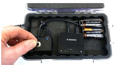
Note: There is a small power switch behind the Avantree Bluetooth box, it should always be in the ON position.
